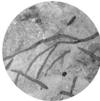
Photomicrograph showing graphite form in gray iron.
